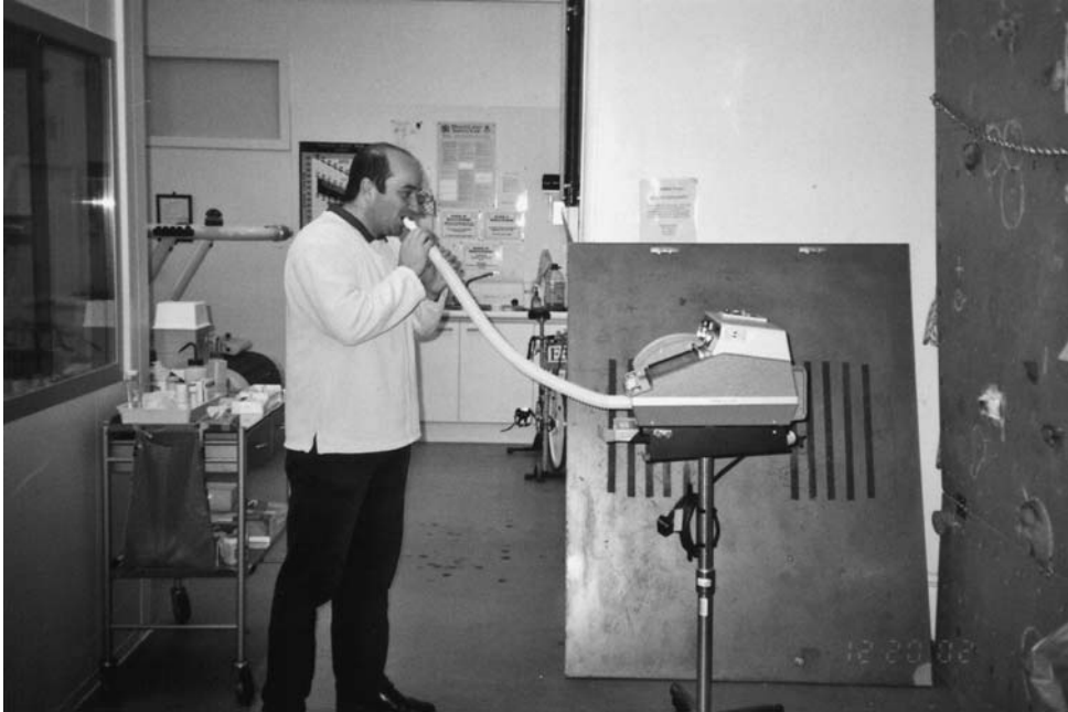
Figure 2.5 The Vitalograph used to record forced expiratory manoeuvres. (Reproduced with permission of University College Chichester)
