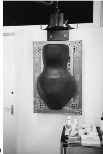
Figure 1.4 Ergometers. (a) A range of ergometers – starting from the right with a treadmill, a cycle ergometer, a rowing ergometer, and on the wall a purpose-built punching ergometer. (b) An isokinetic cycle ergometer. (c) An isokinetic bench for arm, leg and back exercise. (d) Close-up of a sport-specific ergometer for boxing. It consists of a boxing manikin attached to a force platform suspended on a wall. (Reproduced with permission of University College Chichester)
