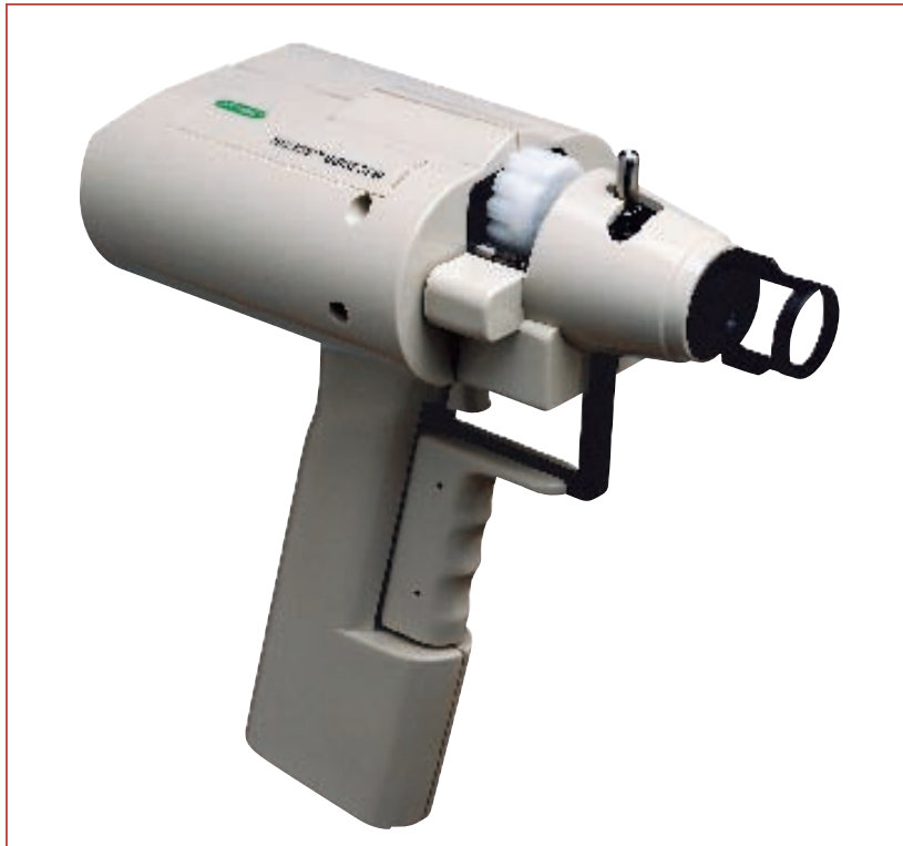
Figure 5.2 A gene gun can be used to inject foreign DNA into a plant cell. The foreign DNA is coated on metal beads and then fired at a collection of plant cells. Once inside the cell, the DNA releases from the bead and becomes incorporated into the plant chromosome.
