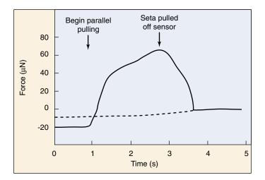
The sliding step experiment. The adhesive force of a single seta was measured. An initial push perpendicularly put the seta in contact with the sensor. Then, with parallel pulling, the force continued to increase over time to a value of 60 microNewtons (after this, the seta began to slide and pulled off the sensor). In a large number of similar experiments, adhesion forces typically approach 200 microNewtons.
