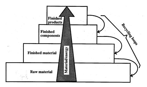
Figure 17.7. A material flow chain or energy/materials pyramid. Less energy and materials are involved when recycling is done near the end of the flow chain, thus retaining embedded utility.
