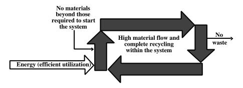
Figure 17.5. Idealized industrial ecosystem in which no materials are required for input beyond those needed to start the system. Energy requirements are relatively high, and the material flow within the system is high and continuous.
