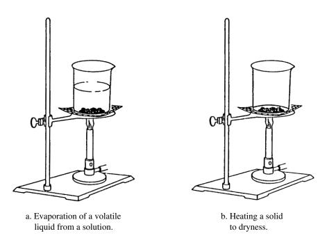
**Figure 4.6** • Assembly for evaporation.
