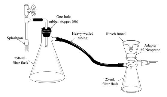
**Figure 31.1** • Vacuum filtration with a Hirsch funnel.
