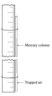
**5.** The length of the column of trapped air is to be measured when the tube is at various angles to the bench top, as outlined in the following table.
