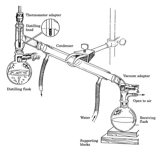
**Figure 5.2** • A distillation apparatus.
