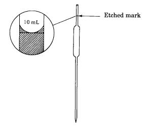
**8.** Drain the liquid from the pipet into a collection flask by pressing valve "E." Remove any drops on the tip by touching the tip of the pipet against the inside walls of the collection flask. Water should remain inside the tip; the pipet is calibrated with this water in the tip.
