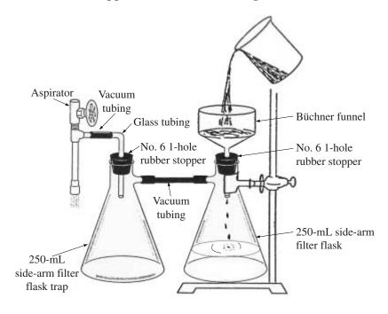
**Figure 6.2** • Vacuum filtration setup using the Büchner funnel.
