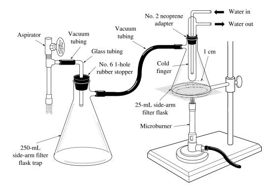
**Figure 37.3** • Sublimation apparatus connected to an aspirator.
