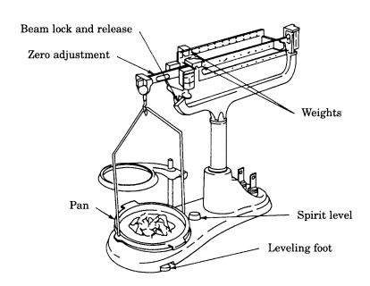
Smaller quantities of material can be weighed on this balance (to a maximum of 311 g). Figure 2.9 illustrates how a reading on this balance would be taken.
