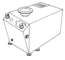
Figure 2.11 Reading on a top loading balance.
