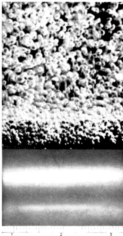
FIG. 14-95a Comparison of bubbles from a porous septum and from a perforated-pipe sparger. Air in water at 70°F. Grade 25 porous-carbon diffuser operating under a pressure differential of 13.7 in of water.
