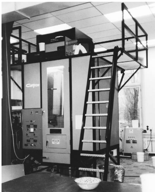
FIG. 19-62 New Triboelectric separator for separation of PVC from other plastics. (Courtesy Carpc, Inc.)
