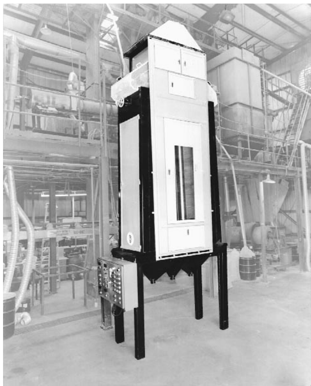
FIG. 19-57 Triboelectric separators. V-Stat electrostatic separator for silica removal from industrial minerals. (Courtesy of Carpc, Inc.)
