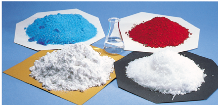
Figure 2-11 One mole of some compounds. The colorless liquid is water, \text{H}_2\text{O} (1 mol = 18.0 g = 18.0 mL). The white solid ( front left ) is anhydrous oxalic acid, (\text{COOH})_2 (1 mol = 90.0 g). The second white solid ( front right ) is hydrated oxalic acid, (\text{COOH})_2 \cdot 2\text{H}_2\text{O} (1 mol = 126.0 g). The blue solid is hydrated copper(II) sulfate, \text{CuSO}_4 \cdot 5\text{H}_2\text{O} (1 mol = 249.7 g). The red solid is mercury(II) oxide (1 mol = 216.6 g).
