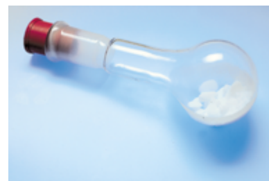
Figure 15-8 A system that absorbs heat at constant volume. Some dry ice [ \text{CO}_2(\text{s}) ] is placed into a rigid flask, which is then sealed. As the dry ice absorbs heat from the surroundings, some \text{CO}_2(\text{s}) sublimates to form \text{CO}_2(\text{g}) . In contrast to the case in Figure 15-6, this system cannot expand ( \Delta V = 0 ), so no work is done, and the pressure in the flask increases. Thus, the heat absorbed at constant volume, q_v , is equal to \Delta E for the process.
