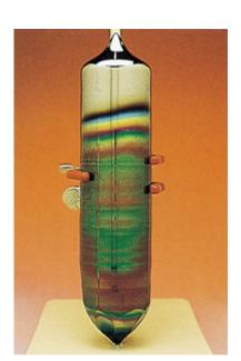
Ultrapure silicon is produced by zone refining.
