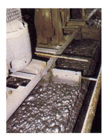
*Figure 22-11* A copper ore being enriched by flotation.
