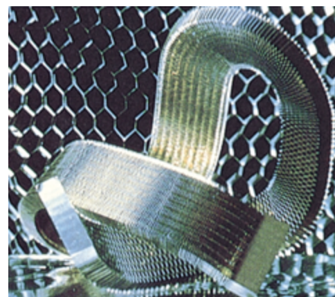
This aluminum honeycomb material is made by bonding aluminum foil sheets to form hexagonal cells. It is used to make sandwich construction panels that have a very high strength-to-weight ratio.
