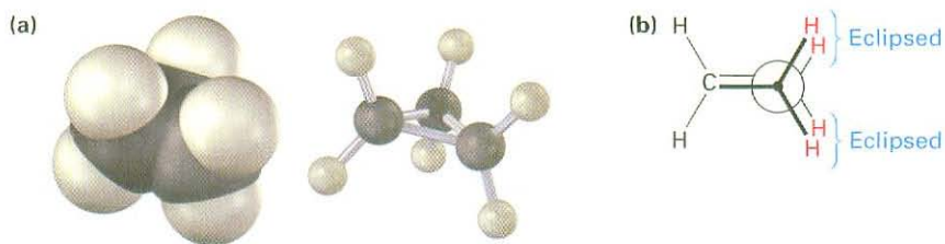
Figure 4.4 The structure of cyclopropane, showing the eclipsing of neighboring C–H bonds that gives rise to torsional strain. Part (b) is a Newman projection along a C–C bond.
