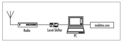
Simple circuitry is needed to convert the audio signal from the radio receiver into the proper levels for computer interfacing. I built the level-shifter hardware—some people call it a *POCSAG decoder* or *Hamcomm interface*—with a few dollars' worth of common components that we had lying around the lab. I plugged one side of it into my laptop's serial port and connected the audio output from the radio into the other side.
