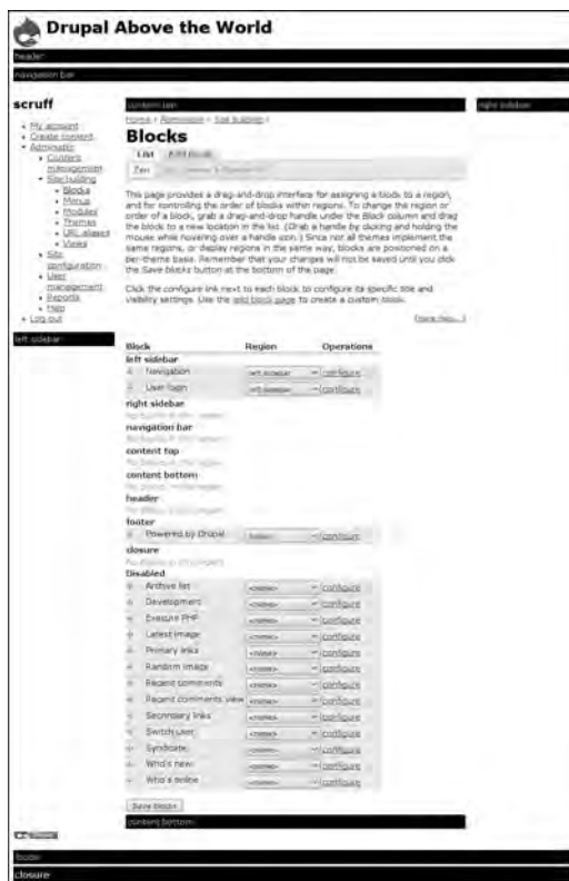
FIGURE 1.12 The Zen theme-building theme comes with eight different regions; they are represented by thick black bars.
