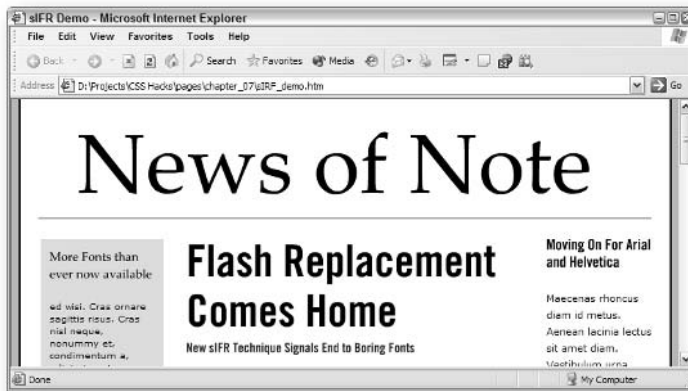
FIGURE 7-15: Each of the headlines here, including the banner, are actually Flash elements, substituted by sIFR.
