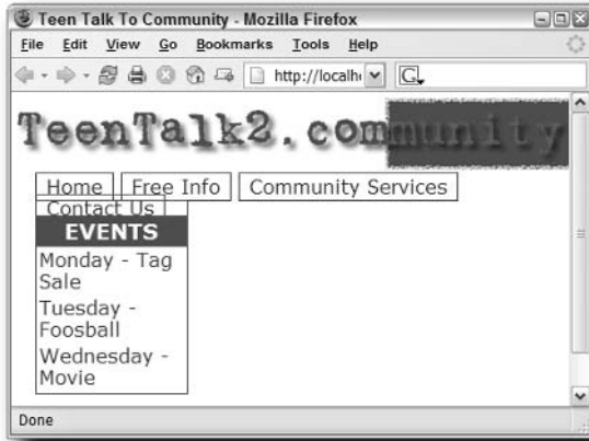
FIGURE 9-5: When an absolutely positioned object is tied to the html tag, undesired overlaps are entirely possible.
