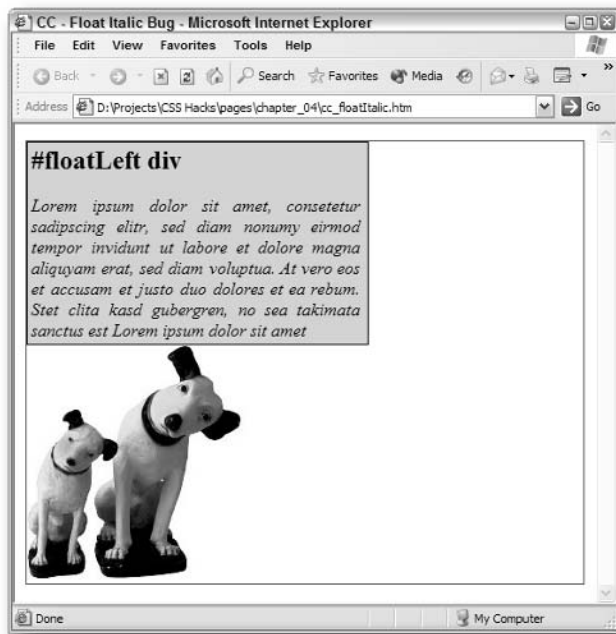
FIGURE 4-5: The italics float bug emerges when a sizable amount of text is italicized; a smaller amount of text can have the same effect if it is also justified.
