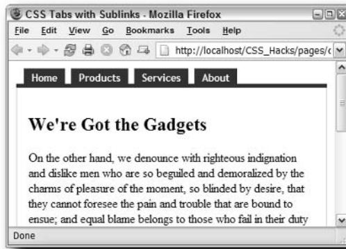
FIGURE 10-7: Combining restyled bulleted list items with a bottom border gives a tab-like appearance.
