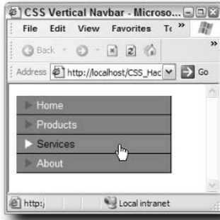
FIGURE 10-3: CSS hacks bring button-like behavior to linked lists, even in Internet Explorer.
