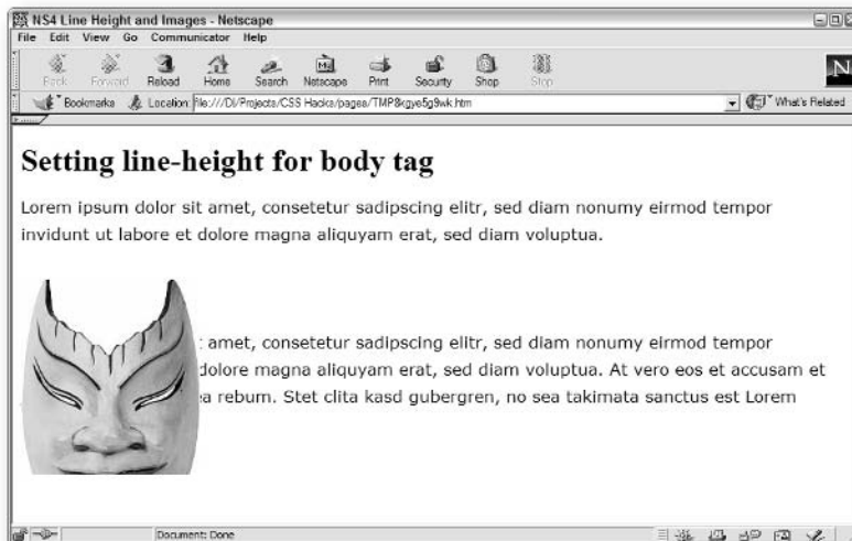
FIGURE 2-8: In a Netscape 4 style sheet, defining line-height declarations in the body property has a disastrous effect on images.
