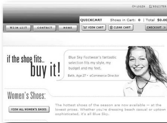
FIGURE 1-4: Internet Explorer 6 is flawed when rendering floated div tags—and the top of the model's head is noticeably off.
