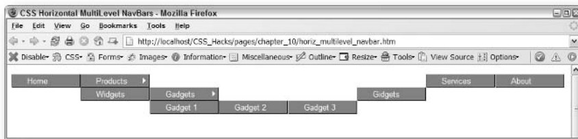
FIGURE 10-5: The navbar is undesirably spread out because the submenus are still visible. Note the parent items with the right-facing triangle.
