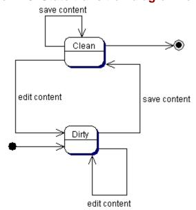
Figure 2.13. State transition diagram for a file
