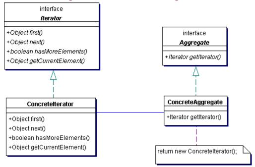
Figure 2.7. Iterator class diagram
