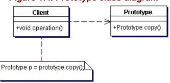
Figure 1.4. Prototype class diagram
