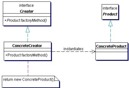
Figure 1.3. Factory Method class diagram
