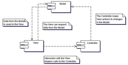
A component diagram has been used to describe this pattern. Each of the three parts of the MVC pattern is a component, that can contain many classes and interfaces.
