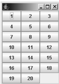
Figure 5-7. You can force GridLayout to use a specific number of columns by specifying a column count but no row count.
