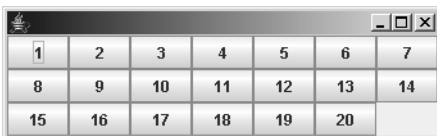
Figure 5-8. You can force GridLayout to use a specific number of rows by specifying a row count but no column count.
