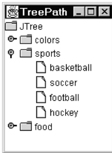
Figure 7-14. To reach the soccer node shown in this tree, you'd need to traverse the JTree , sports , and soccer nodes.
