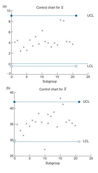
The control charts for  $\overline{X}$  and S with the preceding control limits are shown in Figures 13.2a and 13.2b. Since  $\overline{X}_{10}$  and  $\overline{X}_{15}$  fall outside the  $\overline{X}$  control limits, these subgroups must be eliminated and the control limits recomputed. We leave the necessary computations as an exercise.
