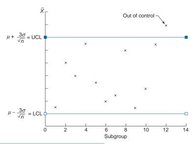
FIGURE 13.1 Control chart for  $\overline{X}$ , n = size of subgroup.
