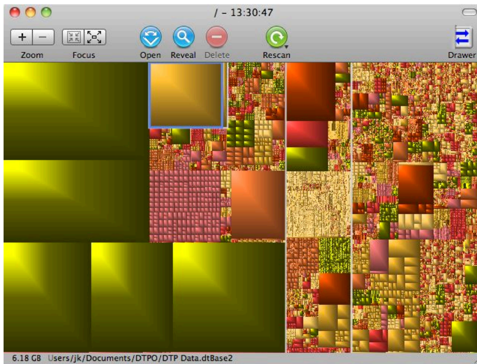
Figure 4: When you can't figure out where all those large files are on your disk, consult a utility such as GrandPerspective.
