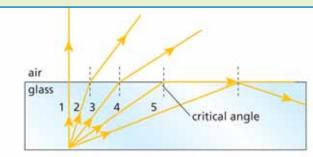
In the diagram, rays 1-3 leave the glass and bend away from the normal as they enter the air. Ray 4 leaves the glass and bends away from the normal such that its angle of refraction is 90°. The angle of incidence is defined as the critical angle. Ray 5 has an angle of incidence greater than the critical angle. It reflects back into the glass. The angle of incidence is equal to the angle of reflection.
