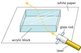
You may notice that some of the incident light is reflected off the acrylic block. Use a series of dots to mark the reflected ray.
