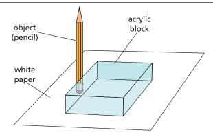
2. Trace the outside of the acrylic block on the paper. Carefully aim a laser pointer, or the light from a ray box, so the light beam moves horizontally, as you did in previous sections. Remember to follow the safety rules when using lasers and never allow any of the transmitted or reflected light to fall on a student's eye.
