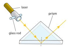
Note that the long side of the prism is acting as a mirror. This situation is called *total internal reflection* because the inside of the prism acts like a perfect mirror (total reflection) and the reflected light stays inside the prism (until it gets to the other side).
