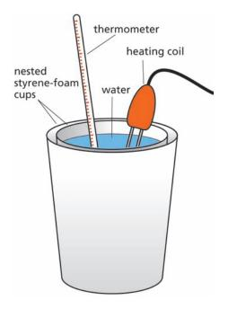
2. Note the time at which you begin sending electric current through the resistor. Keep the electric heater operating for the amount of time recommended by your teacher. When you stop the current, note the time, stir the water, and measure the final, maximum temperature of the water.
