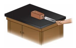
5. Continue adding sand to increase the weight of the box to 4.0, 6.0, 8.0, and 10.0 N, recording the newton force reading of the pull of the spring scale for each weight of the box.
