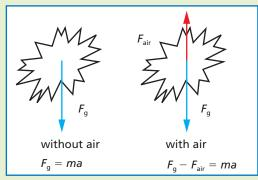
Notice that the acceleration with air will be smaller since the force due to air resistance opposes the gravitational force.
