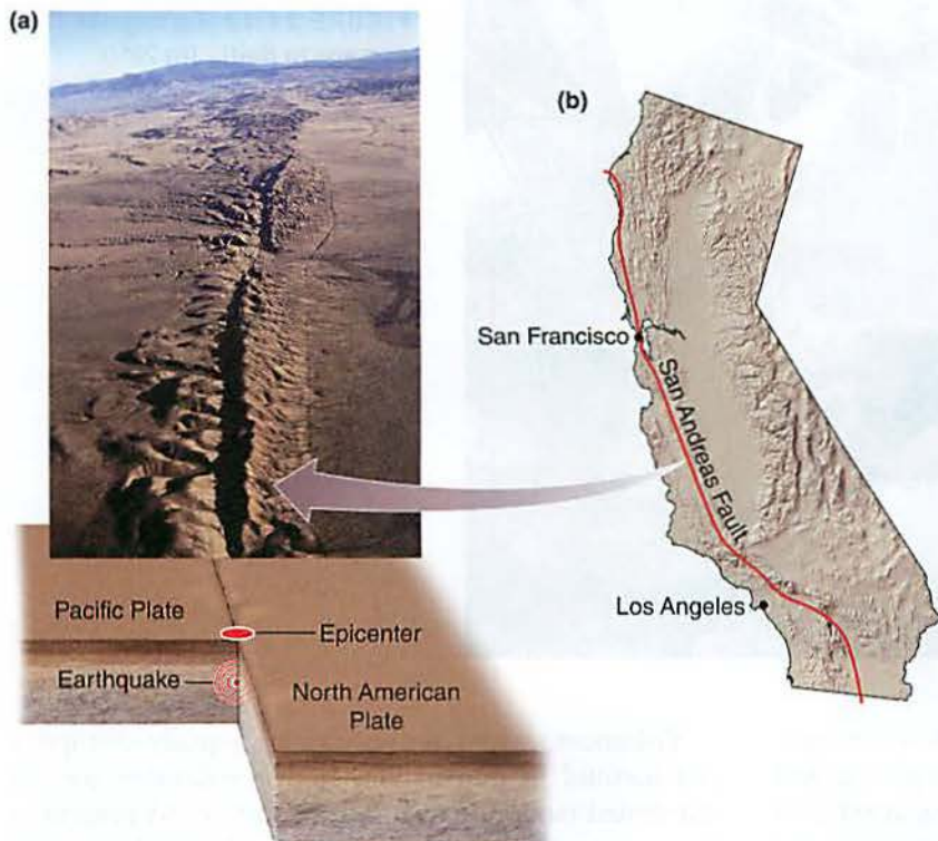
FIGURE 24.10 A fault zone. Many areas of seismic activity, including the San Andreas Fault in California, are characterized by a transform fault. The epicenter of an earthquake is the point on the surface of Earth directly above the location where the rock ruptures. (age fotostock/SuperStock)
