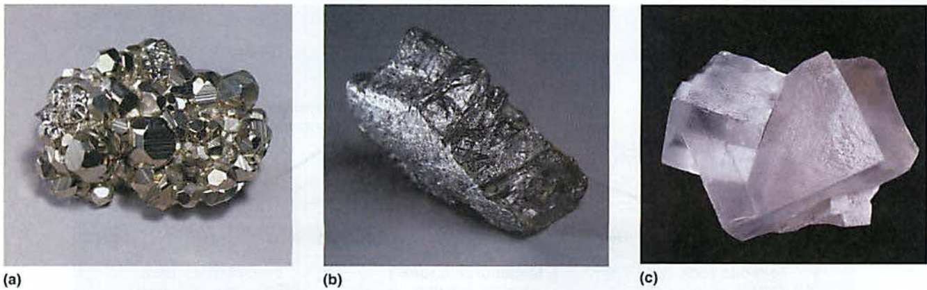
FIGURE 24.14 Some common minerals. (a) Pyrite ( \text{FeS}_2 ), also called “fool’s gold.” (b) Graphite, a form of carbon (C). (c) Halite, or table salt ( \text{NaCl} ). (a–b: John Grotzinger/Ramón Rivera-Morel/Harvard Mineralogical Museum; c: The Natural History Museum/Alamy)
