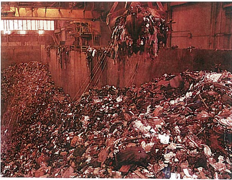
FIGURE 9.18 Waste to Energy Municipal trash can be burned to produce heat and electricity. This refuse pit is used to feed hoppers of high-temperature furnaces.
