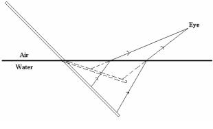
13. The light rays leaving the fish bend away from the normal as they exit the tank and go into your eye. Thus, you see the image of the fish "above" (in this figure) the position of the real fish. Also, the image appears to be slightly closer to the wall of the aquarium. Since your brain doesn't know that light bends at the water/air interface, when your brain "follows" the ray back into the tank, it interprets the location of the fish as above its actual location.
