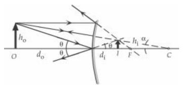
21. (a) To produce a smaller image located behind the surface of the mirror requires a convex mirror.(b) We find the image distance from the magnification:
