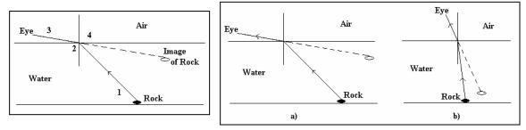
12. Your brain interprets the bending rays as if that the part of the stick that is underwater is shallower than it really is, so it looks bent. Each point on the stick that is underwater appears to you to be closer to the surface than it actually is.
