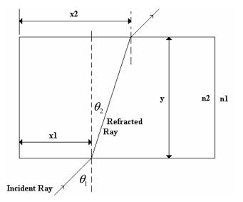
find the index of refraction of the block:  $n_2 = n_1 \frac{\sin \theta_1}{\sin \theta_2}$ . The index of refraction for air  $(n_1)$  is basically
