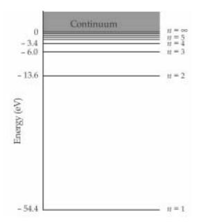
58. Doubly ionized lithium is like hydrogen, except that there are three positive charges (Z = 3) in the nucleus. The square of the product of the positive and negative charges appears in the energy term for the energy levels. We can use the results for hydrogen, if we replace  $e^2$  by  $Ze^2$ :
