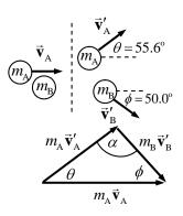
The collision is elastic, so write the KE conservation equation, and substitute the results from above. Also note that  $\alpha = 180.0 - 55.6^{\circ} - 50.0^{\circ} = 74.4^{\circ}$
