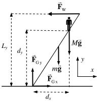
have a maximum counterclockwise torque that it can exert. As the person climbs the ladder, their lever arm gets longer and so the torque due to their weight gets larger. Eventually, if the torque caused by the person is larger than the maximum torque caused by  $\vec{F}_w$ , the ladder will start to slip – it will not stay in equilibrium.
