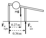
23. (*a*) The meter stick is in equilibrium, so the net torque and the net force are both zero. From the force diagram, write an expression for the net torque about the 90-cm mark, with counterclockwise torques as positive.
