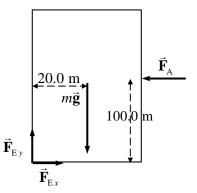
Since this is a negative torque, the building will tend to rotate clockwise, which means it will rotate back down to the ground. Thus the building will not topple .
