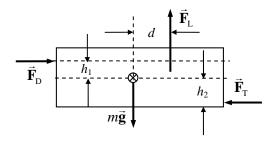
Calculate the torques about the CM, calling counterclockwise torques positive.
