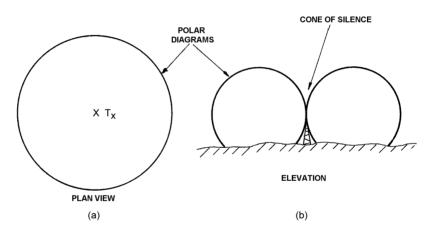
58. It is equally convenient to produce polar diagrams for receiver aerial arrays. Now the situation is reversed in that a signal of a given strength which is transmitted from any point on the polar diagram will induce a current of constant amplitude to flow in the receiver aerial.
