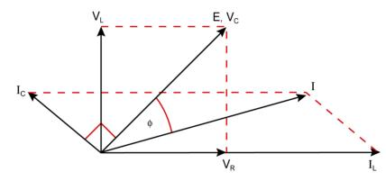
50. For a certain value of frequency, I is in phase with E, i.e. the circuit is at RESONANCE. Once again it can be shown that the value of the Resonant Frequency  $(F_O)$  is given by:
