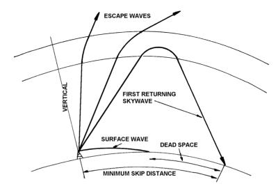
97. The preceding diagrams have shown only **single hop sky waves**. Providing that the signal has sufficient power there is no reason why it should not make the return journey to the Earth's surface via the ionosphere two or even three times. This is known as **multi-hop propagation**.
