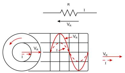
37. An ac flows through a resistance of R ohms, see Figure 1-11. From ohms law we know that  $V_R$  = IR. Thus for a pure resistance, the potential difference across it,  $V_R$ , is IN PHASE with the current flow through it.
