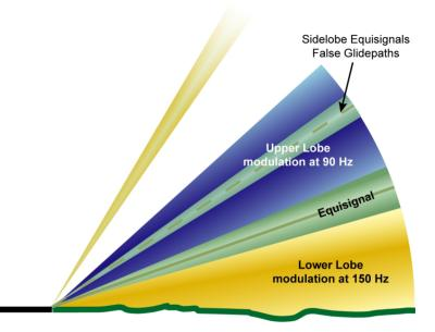
200. Glidepath coverage in azimuth (for United Kingdom installations) is provided through an arc of  $8^{\circ}$  on either side of the localiser centreline out to a range of 10 nm from the threshold, as illustrated at Figure 1-68.
