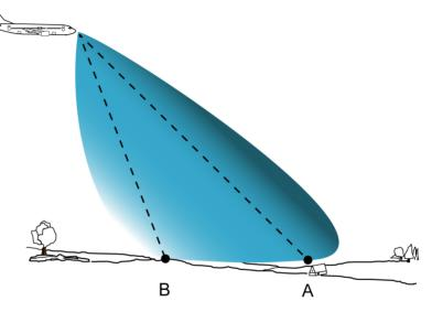
180. This specialised type of pattern is often produced by distorting the upper portion of a parabolic reflector, so that more energy is directed at the longer range targets than towards those at short range (Figure 1-58).
