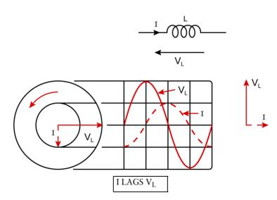
**Inductive Reactance.** In a pure resistance the ratio of voltage to current gives the resistance R. In a pure inductance the ratio of voltage to current is:
