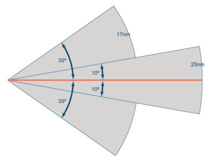
194. In the United Kingdom ILS localisers which are associated with steep angle glidepath transmitters provide coverage from the centre of the localiser antenna to distances of:
