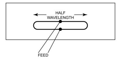
Some types of aircraft suppressed aerial are based on the slot. In these aerials, the slot is cut 168. in the aircraft skin. Half-wave slots cut in the wall of a waveguide, feature in the design of certain microwave aerials.
