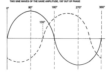
FIGURE 1-5 Two Sine Waves, 135° Phase Difference
