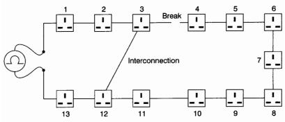
Figure 17 Ring circuit with inferconnection
