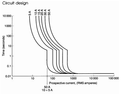
**Figure 36** Time/current characteristics for type 3 CBs to BS EN 60898 and RCBO's. Example for 50 A superimposed. For times less than 20 ms, the manufacturer should be consulted
