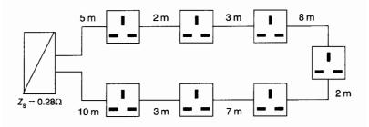
MCB. If a test for continuity was performed at 15°C using the measurement at each socket method, calculate:
