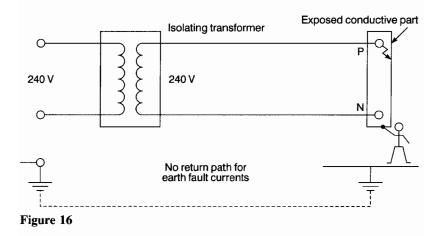
earth exposed conductive parts such as small fixings, screws and rivets, provided that they cannot be touched or gripped by a major part of the human body (not less than 50 mm by 50 mm), and that it is difficult to make and maintain an earth connection.
