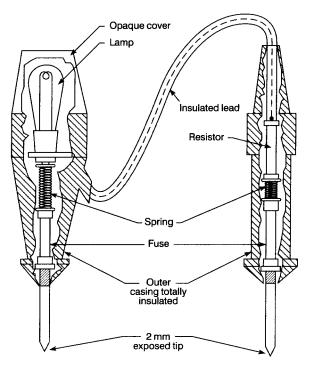
Figure 16 Approved test lamp
