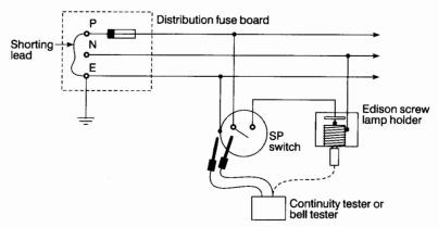
Figure 32 Polarity test on lighting circuit
