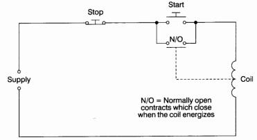
Figure 21 Hold-on circuit
