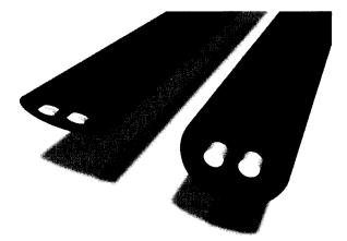
**Figure 15** Mineral-insulated cable. On impact, all parts including the conductors are flattened, and a proportionate thickness of insulation remains between conductors, and conductors and sheath, without impairing the performance of the cable at normal working voltages
