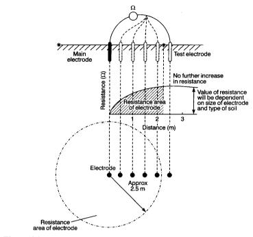
Testing earth electrode resistance
