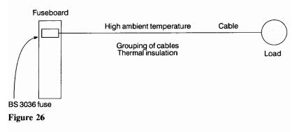
logical to apply all the CFs, as they all affect the whole cable run. Certainly the factors for the BS 3036 fuse, grouping and thermal insulation should be used. However, it is doubtful if the ambient temperature will have any effect on the cable, as the thermal insulation, if it is efficient, will prevent heat reaching the cable. Hence, apply  $C_g$ ,  $C_f$  and  $C_i$ .
