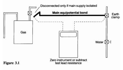
the resistance of parallel paths of other earthed metalwork. Remember to zero the instrument first or, if this facility is not available, record the resistance of the test leads so that this value can be subtracted from the test reading.
