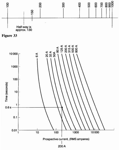
Figure 34 Time/current characteristics for fuses to BS 88 Part 2. Example for 32 A fuse superimposed
