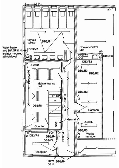
Figure 12 Example floor plan
