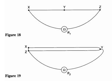
In order to apply this principle to a ring final circuit, it is necessary to know the position of the socket nearest the mid-point of the ring. The test procedure is then as follows for each of the conductors of the ring:
