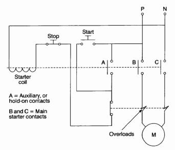
Figure 22 Single-phase motor starter
