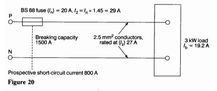
prospective short-circuit current (PSCC) at the point of installation, it will also protect against short-circuit currents. However, if there is any doubt the formula should be used.
