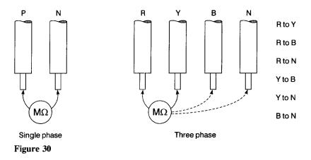
For small installations, the tests are performed on the whole system, whereas for larger complex types, the installation may be sub-divided into sections and tests performed on each section. The reason for this is that as conductor insulation and the circuits they supply are all in parallel, a test on the whole of a large installation would produce pessimistically low readings even though no faults exist.
