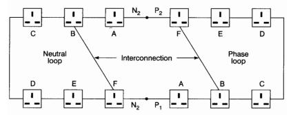
Figure 26 Healthy ring with interconnection. Sockets A, B and F will give identical readings. C, E and D will not.
