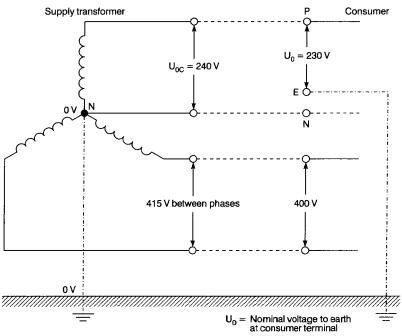
Note: The connection of the transformer star or neutral point to earth, helps to maintain that point at or very near zero volts.
