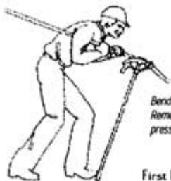
FIGURE 5.22 Techniques for bending conduit. (Courtesy Ideal Industries, Inc.)
