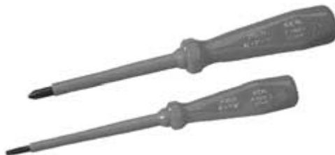
FIGURE 11.5 Insulated electrician's screwdrivers.
