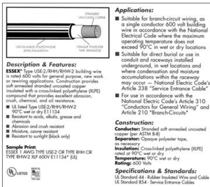
FIGURE 10.18 Type USE-2/Rhh/RhW-2 single conductor description and application. (Courtesy Superior Essex)
