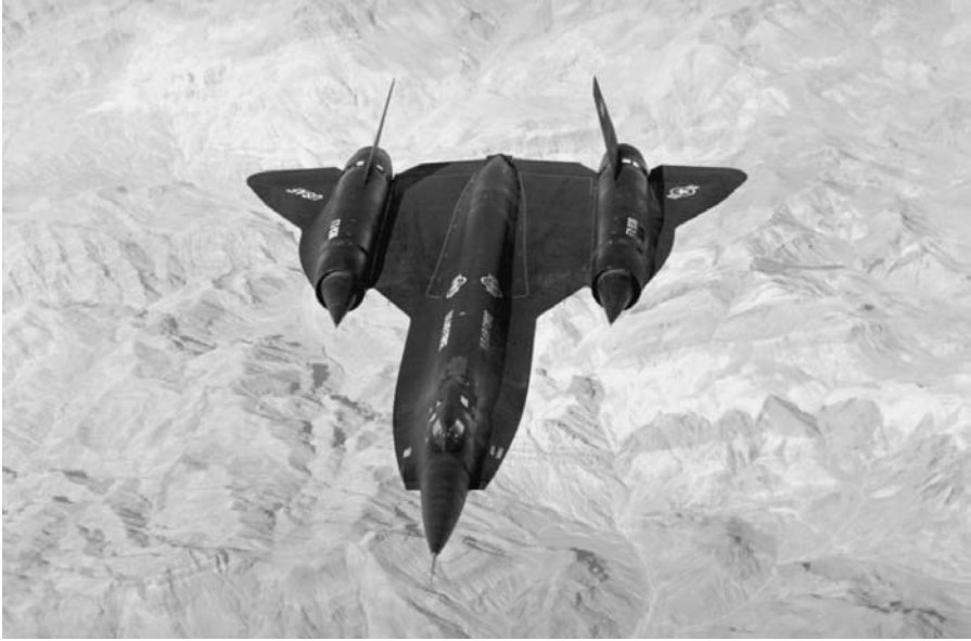
Figure 7.17 YF-12 plane showing conical air inlets. (Lockheed Martin photo.)
