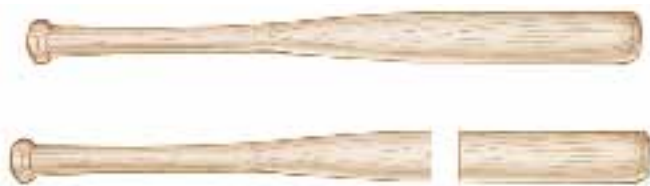
Figure 9.21 A baseball bat cut at the location of its center of mass.
