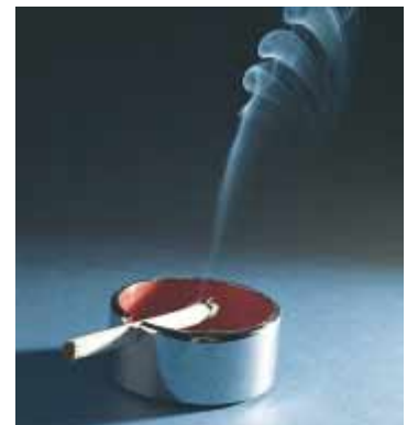
Figure 15.15 Hot gases from a cigarette made visible by smoke particles. The smoke first moves in laminar flow at the bottom and then in turbulent flow above.
