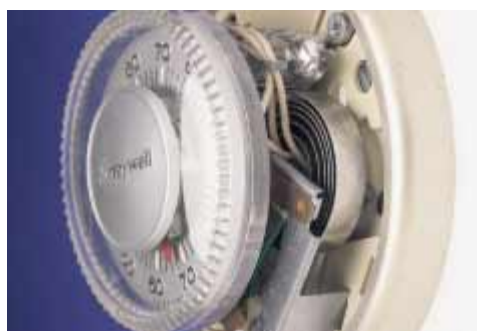
Figure 19.9 (a) A bimetallic strip bends as the temperature changes because the two metals have different expansion coefficients. (b) A bimetallic strip used in a thermostat to break or make electrical contact. (c) The interior of a thermostat, showing the coiled bimetallic strip. Why do you suppose the strip is coiled?
