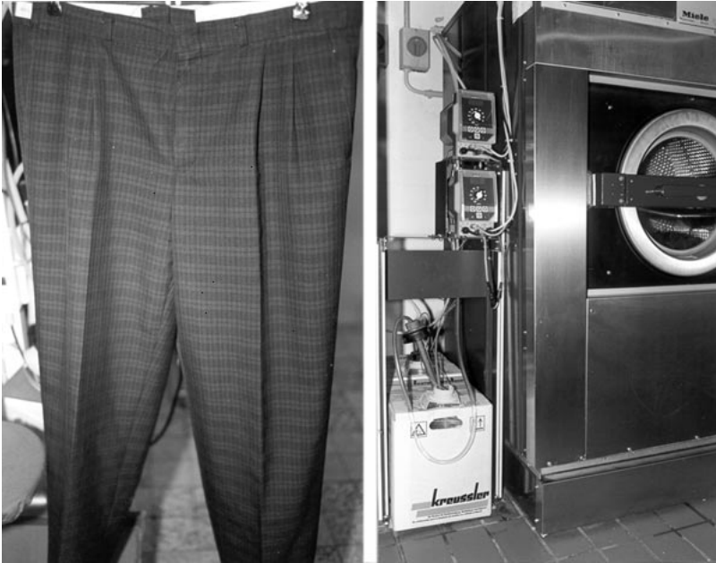
Figure 21.4.2. (left) Polyester/wool trousers after drying.(right) Dosing method for polyester/wool trousers after drying LANADOL AKTIV and LANADOL APRET.
