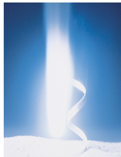
Figure 1-1 Magnesium burns in the oxygen of the air to form magnesium oxide, a white solid. The mass of magnesium oxide formed is equal to the sum of the masses of oxygen and magnesium that formed it.
