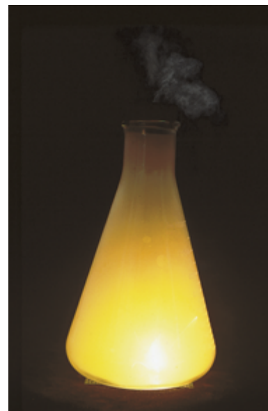
Figure 1-10 The reaction of sodium, a solid element, and chlorine, a gaseous element, to produce sodium chloride (table salt). This reaction gives off considerable energy in the form of heat and light.
