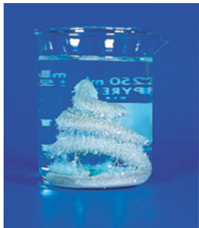
Metallic silver formed by immersing a spiral of copper wire in a silver nitrate solution (see Example 4-4a).
