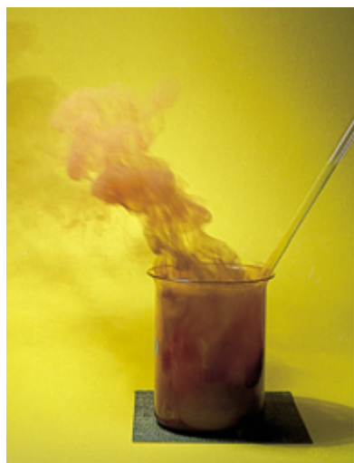
Iron reacting with chlorine to form iron(III) chloride.
