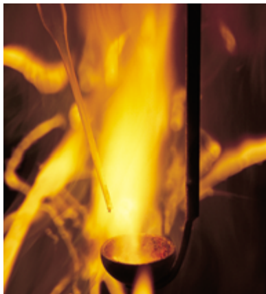
Phosphorus and chlorine, two nonmetals, react to form phosphorus pentachloride, \text{PCl}_5 .
