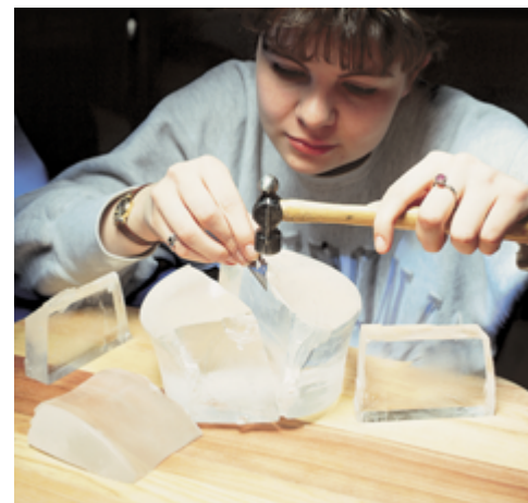
A crystal can be cleaved into smaller crystals that have the same appearance as the larger crystal. Here a worker is cleaving a large crystal of sodium chloride.
