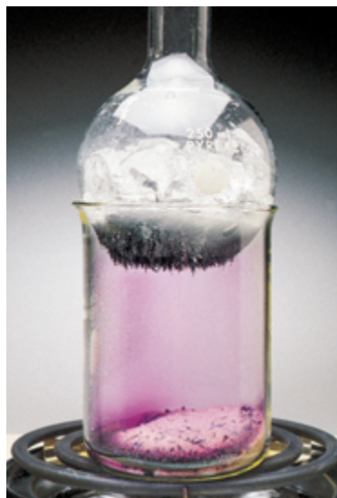
Figure 13-16 Sublimation can be used to purify volatile solids. The high vapor pressure of the solid substance causes it to sublime when heated. Crystals of purified substance are formed when the vapor is deposited to form solid on the cooler (upper) portion of the apparatus. Iodine, \text{I}_2 , sublimes readily. \text{I}_2 vapor is purple.
