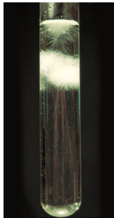
A tiny crystal of sodium acetate, \text{NaCH}_3\text{COO} , was added to a clear, colorless, supersaturated solution of \text{NaCH}_3\text{COO} . This photo shows solid \text{NaCH}_3\text{COO} just beginning to crystallize in a very rapid process.
