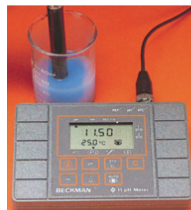
Measurement of the pH of a solution of household ammonia.
