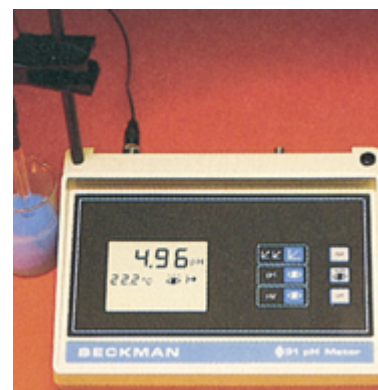
The pH of 0.20 M \text{NH}_4\text{NO}_3 solution is 4.96.
