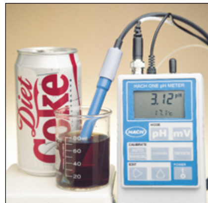
The pH of a soft drink is measured with a modern pH meter. Many soft drinks are quite acidic due to the dissolved \text{CO}_2 and other ingredients.
