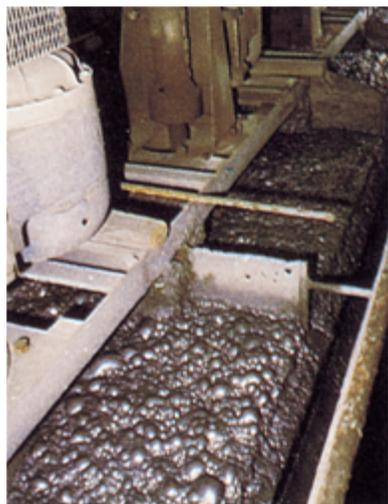
**Figure 22-11** A copper ore being enriched by flotation.
