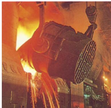
Molten steel is poured from a basic oxygen furnace.
