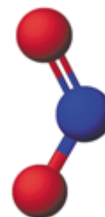
Nitrogen dioxide, \text{NO}_2 , mp -11.20^{\circ}\text{C} , one unpaired electron, bond length 1.197 \text{ \AA} ; brown gas.
