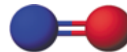
Nitrogen oxide, or nitric oxide, NO, mp -163.6^{\circ}\text{C} , bp -151.8^{\circ}\text{C} , bond distance ( 1.15 \text{ \AA} ) intermediate between \text{N}\equiv\text{O} ( 1.06 \text{ \AA} ) and \text{N}=\text{O} ( 1.20 \text{ \AA} ).
