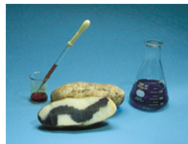
Iodine reacts with starch (as in this potato) to form a deep-blue complex substance.
