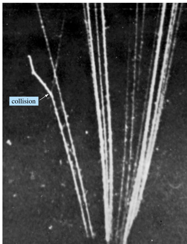
Figure 26-3 A cloud chamber. The emitter is glued onto a pin stuck into a stopper that is mounted on the chamber wall. The chamber has some volatile liquid in the bottom and rests on dry ice. The cool air near the bottom becomes supersaturated with vapor. When an emission speeds through this vapor, ions are produced. These ions serve as “seeds” about which the vapor condenses, forming tiny droplets, or fog.
