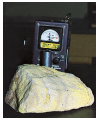
A sample of carnotite, a uranium ore, shown with a Geiger–Müller counter.
