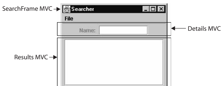
Figure 15.2 The MVC structure of the search application.
