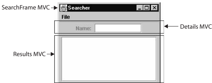
Figure 16.2 The MVC structure of the search application.
