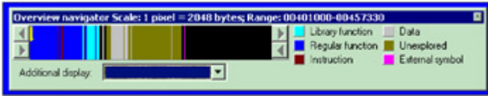
Figure 14: The structure of pkzip.exe , showing all library functions in one place — at the end of the code segment, but before the beginning of the data segment
