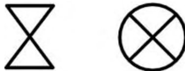
Figure 11.15. Two UML 2.0 symbols for activity diagrams. The one on the left models the passage of time. The one on the right shows the end of a specific sequence of activities.
