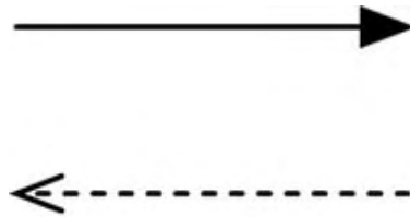
Figure 9.2. The UML symbol for a call and for a return.
