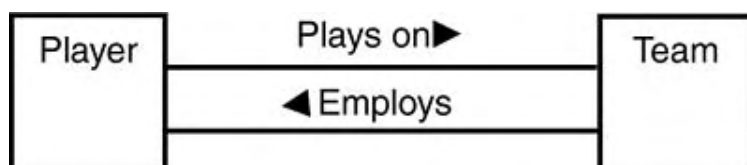
Figure 4.3. Two associations between classes can appear on the same diagram.
