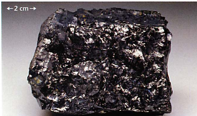
Figure 2.25 Anthracite coal, often called hard coal, forms from the metamorphism of bituminous coal.
