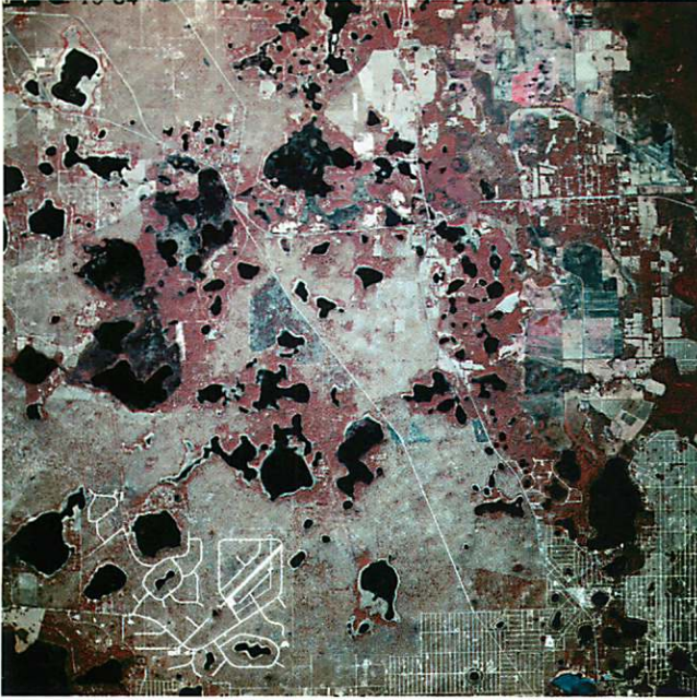
Figure 4.22 This high-altitude infrared image shows an area of karst topography in central Florida. The numerous lakes occupy sinkholes. (Courtesy of USDA-ASCS)
